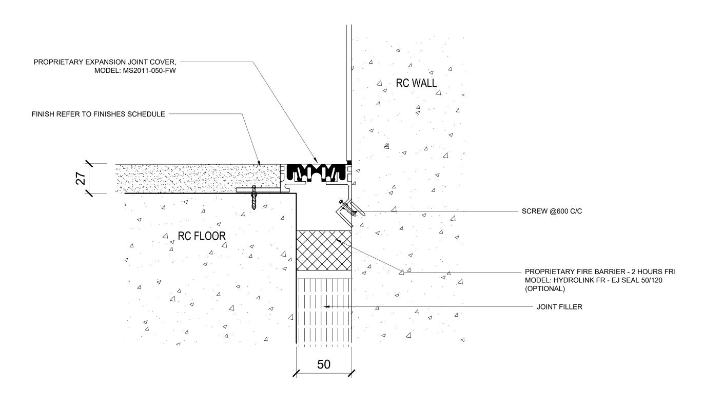
PROPRIETARY FLUSH TINE LINE MOVEMENT JOINT COVER DETAIL FOR INTERNAL FLOOR (FLOOR TO WALL)
