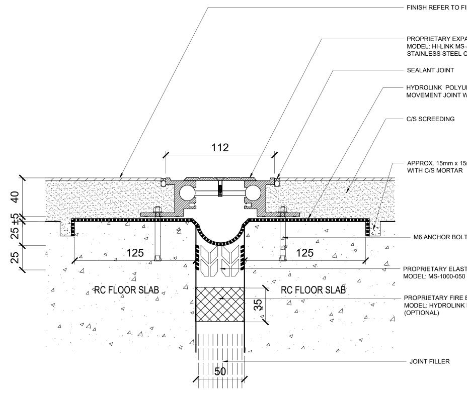
PROPRIETARY METAL MOVEMENT JOINT COVER DETAIL MODEL NO.: HI-LINK MS-4000-50 (FLOOR TO FLOOR)
