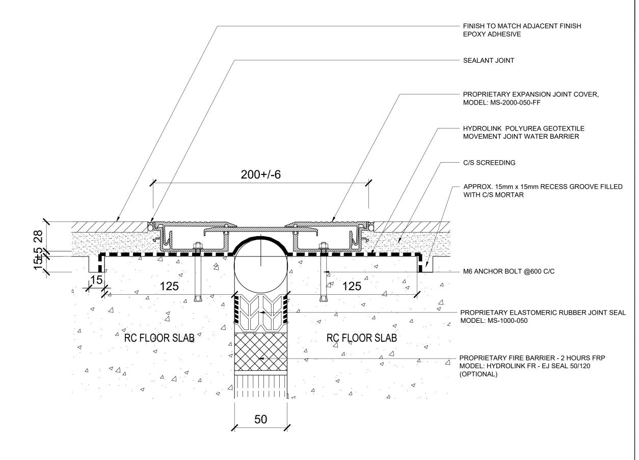
PROPRIETARY SEISMIC LOCK METAL MOVEMENT JOINT COVER SYSTEM MODEL NO.: HI-LINK MS-3000-50 (FLOOR TO FLOOR)
